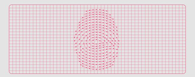
**CAPACITIVE** - Generates the fingerprint image by passing a small electrical current across the surface of the finger.
