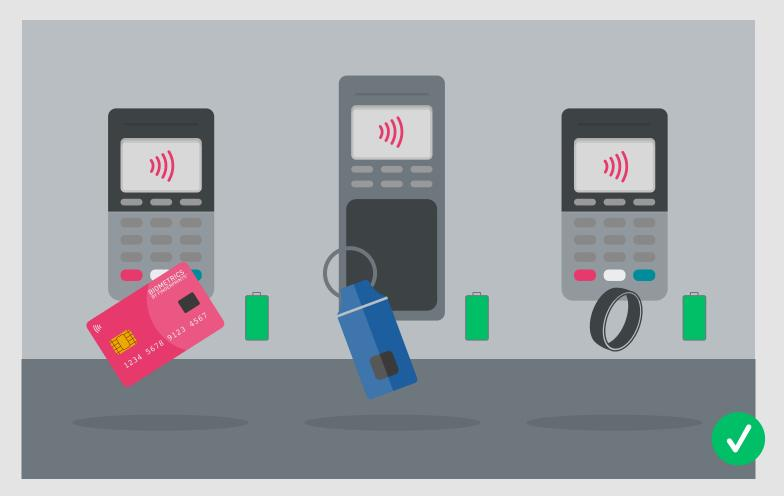
For payments cards, ultra-low power sensors are able to operate on the energy harvested from the POS terminal and the NFC field in the same way contactless cards are powered today. This same ultra-low power technology is being utilized for other contactless use cases too, such as access control cards, small fobs and rings.
